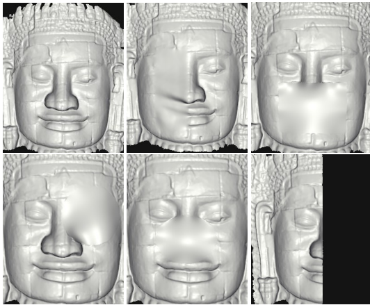
Figure 7: Examples of synthesized data. Upper left: the original shape. The rest: synthesized samples, generated by cutting down a certain facial area randomly, as illustrated in Figure 7. Holes are filled using simple smooth surface.
